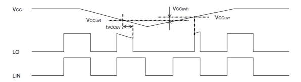
If  $V_{CC}$  supply voltage drops below UV trip voltage ( $V_{CCuvt} = V_{CCuvr} - V_{CCuvh}$ ) for  $V_{CC}$  supply UV filter time, output signal becomes "L". As soon as  $V_{CC}$  supply voltage rises over UV reset voltage, output signal HO becomes "H" it input signal is "H". ( $V_{CC} > V_{BS}$ )
